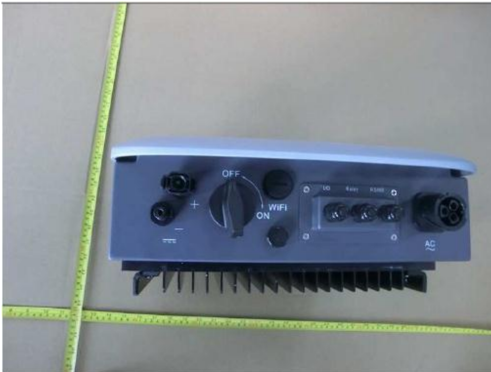
Connection interface of the unit
